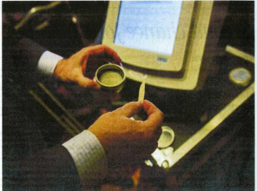
A demonstration of Implant Sciences' QS-B220, the first non-radioactive explosives trace detector approved for screening purposes at United States airports. A sensor is an important component in such a device. AFP pic
